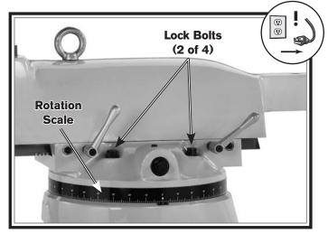
Figure 32. Ram rotating controls.
